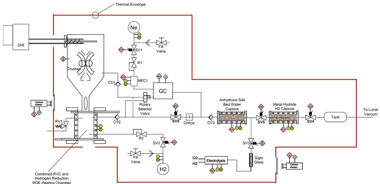
**FIGURE 6.** Conceptual Integrated RESOLVE unit
